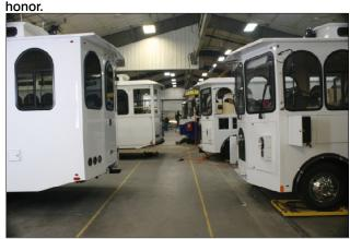
Trolleys under construction on the assembly line. Custom paint will follow.
